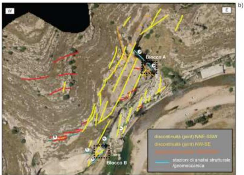
**Figure 2.** a) Satellite photograph of the area; b) Structural plan map of the area under study, showing main joint systems, position of structural analysis stations 1-7 and rock masses-blocks A and B.
