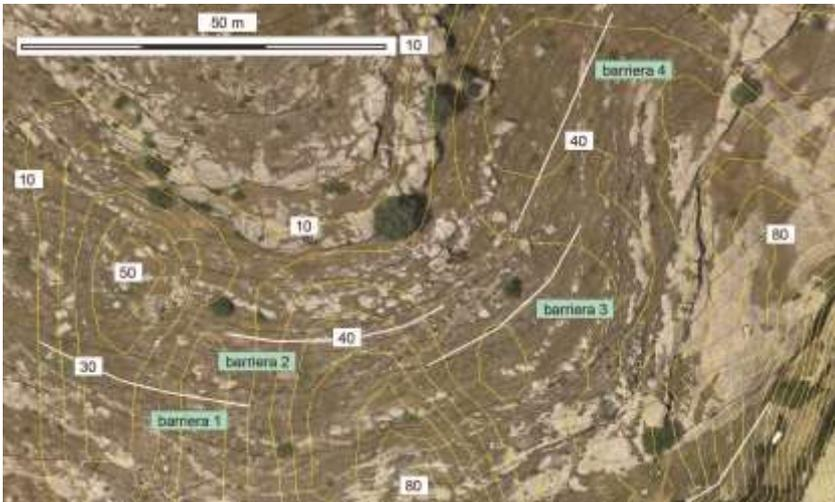
**Figure 31.** Proposed positions for the rockfall barriers based on specific Ecin values.
