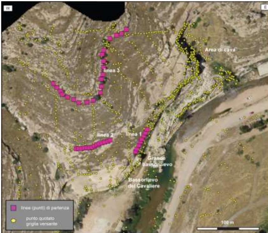
**Figure 11.** Representation of the starting lines and points of the rockfall simulations (lines 1-3) and positions-distributions of topographic grid points measured in the field.
